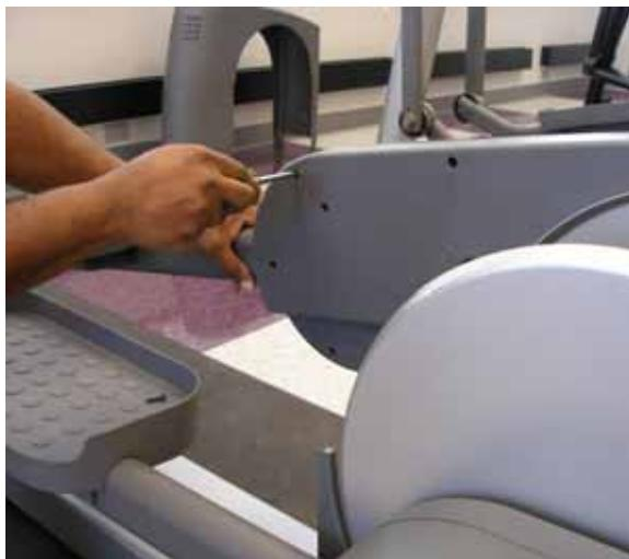
Fig. 3: loosening the right outer link cover screws
