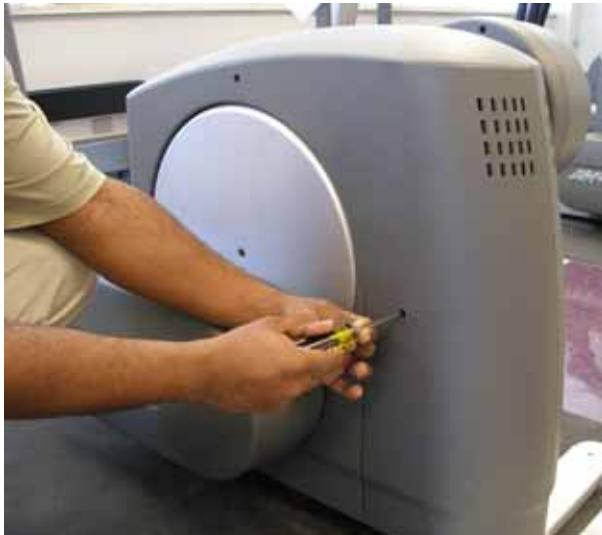
Fig. 1: loosening the main shroud screws
