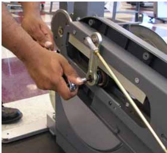
Fig. 5: removing the crank extension bolt
