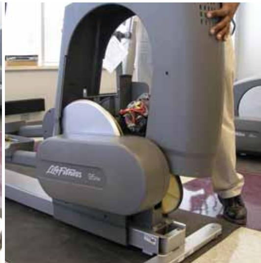
Fig. 2: removing the main shroud
