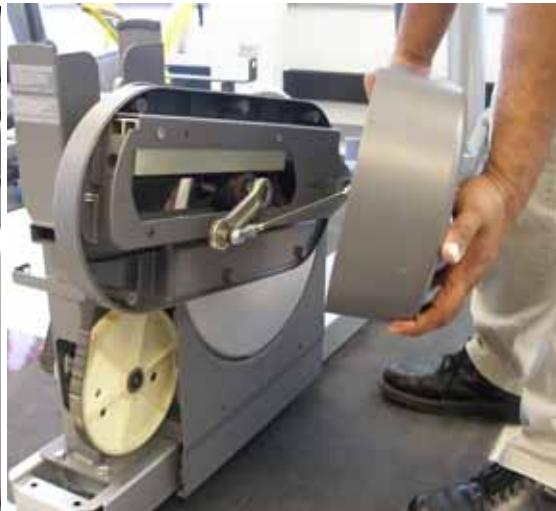
Fig. 4: removing the right outer link cover
