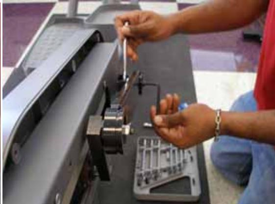
Fig. 8: installing the new control link assembly
