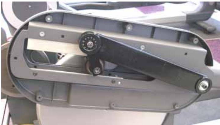
Fig. 10: new control link assembly installed.
